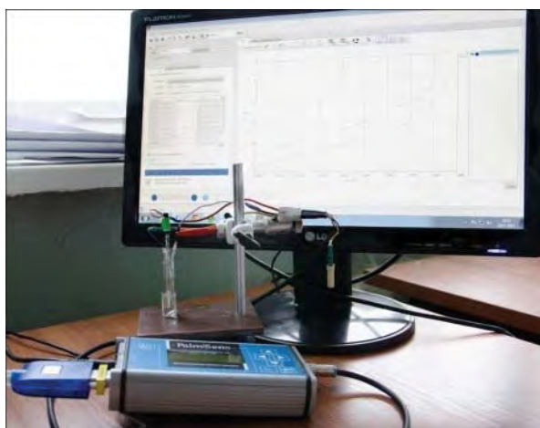
Fig. 1. General view of the biosensor setup (potentiostat, working cell with three electrodes, and computer)
