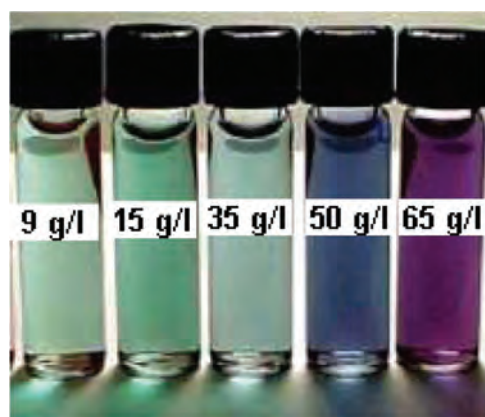
Fig. 5. Appearance of colloidal solutions with different concentration of precursor — encapsulated copper nanopowder
